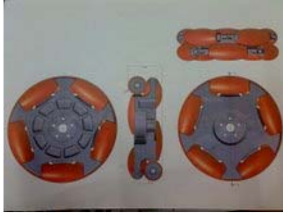
Fig. 3 – Minho team new developed omnidireccional wheels
