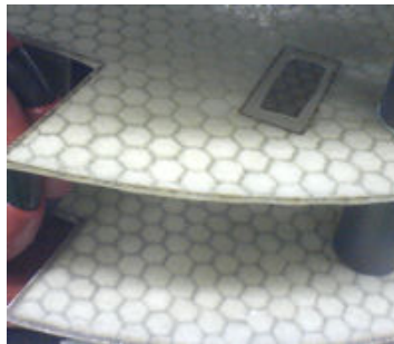
Fig. 2 – Fibreglass sandwich boards – layer 0 and layer 1
