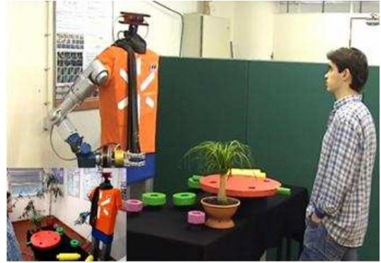
Figure 1. Human-robot team for the joint construction of a toy 'vehicle'. The vehicle consists of a (red) round platform with an axle where two (green) wheels have to be mounted and fixed with (magenta) bolts.
