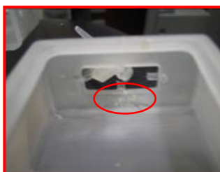
Fig. 13. Vestiges of SL resin in the mouldings
