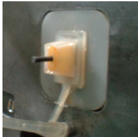
Figure 2.18 - PET moulding perforated by the ejector pin (source: Gonçalves et al. [93])
