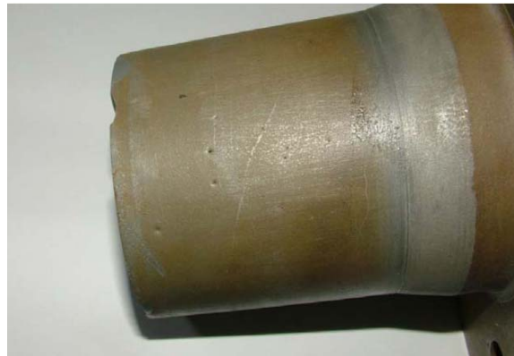
Figure 2.14 – Failure of the epoxy/Al core moulding surface (source: Baretta [95])
