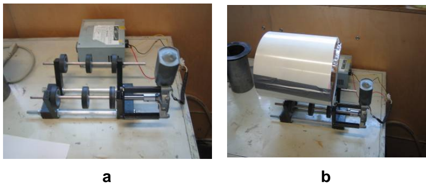
Figure 4.20 - Anti-sedimentation equipment: a) overall view, b) equipment in operation
