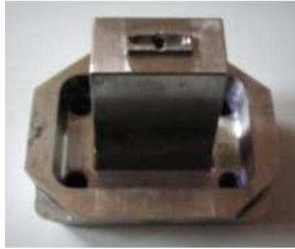
Figure 4.15 - HM-2 steel core used as master
