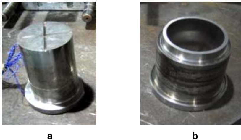
Figure 4.14 – HM-1 steel moulding blocks used as masters: a) core, b) cavity
