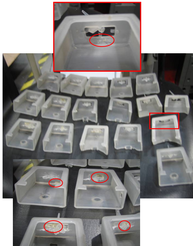
Figure 5.45 - Residues of SL resin in the mouldings
