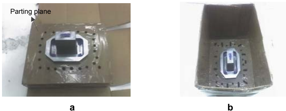
Figure 4.17 - Structure for silicone casting: a) Parting plane definition and holed for silicone cast, b) Structure ready for casting
