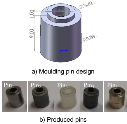
Fig. 4. Moulding pins: a) CAD model b) as used on experimental tests
