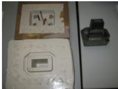
Figure 4.18 - Silicone mould and master
