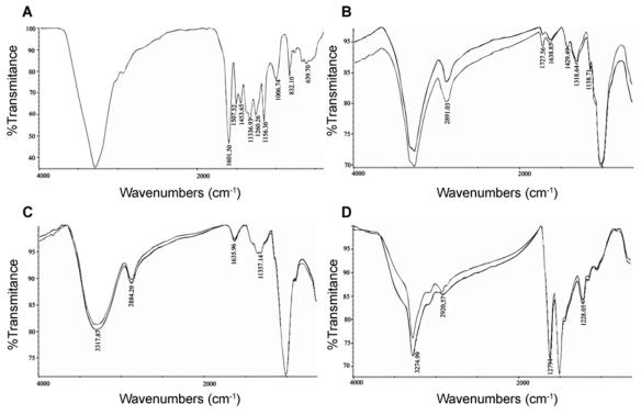
Figure 1. FTIR-ATR Spectra of the Res (KBr capsule) (A), the Res-cotton (B), Res-bamboo (C), and the Res-silk (D). The lither line is the fabric without Res and the darker line is the fabric with Res.
