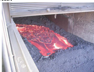
Figure 2 - Emptying of steel slag at the end of the oxidation phase.
