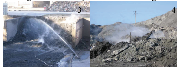
Figures 3 e 4 - Cooling of steel slag with water (3) and to air (4).
