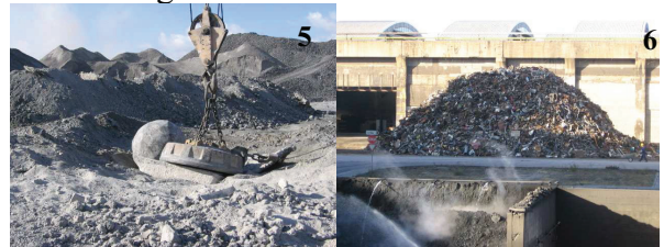
Figures 5 e 6 –Breaking up equipment of steel slag (5) and metallic parts recovered during the processing (6).
