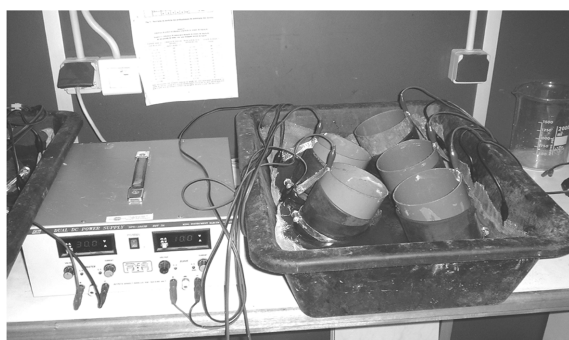
Fig. 1 Test of penetration of chlorides.
