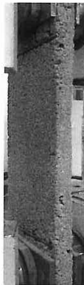
Figure 3.2 – Specimen of mortar reinforced with EMS mounted on the testing machine.
