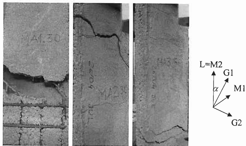
Figure 3.5 – Crack patterns and failure mode of the mortar specimens reinforced with EMS at 30°.
