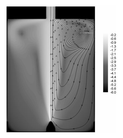
Fig. 6. Contour-plot of the logarithm of the modulus of the total velocity (normalized to its maximum value), numerically calculated for the AIT-reactor represented in Fig. 1, adopting the hollow radial profile of the electron density [see Fig. 2(a)] at  $n_{\rm e,max} = 10^{15} {\rm cm}^{-3}$ ,  $Q = 10^3 {\rm sccm}$ , and  $T_{g_w} = 300 {\rm K}$ . The gradients of grey in background are for the intensity of  $\mathbf{v}$ , whereas the streamlines are for its direction.
