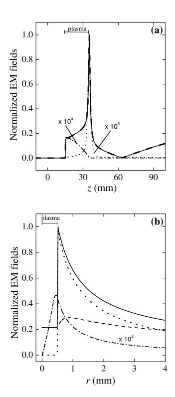
Fig. 4. Calculated axial (at  $r=0^+$ ) (a) and radial (at  $z=l_n^+$ ) (b) profiles of the modulus of the EM field components (normalized to the maximum of the total electric field E) near the plasma region, obtained adopting the hollow radial profile of the electron density [see Fig. 2(a)] at  $n_{\rm e,max}=10^{15}~{\rm cm}^{-3}$ . Results are for the following field components: E (solid curves),  $E_z$  (dashed),  $E_r$  (dotted),  $H_\varphi$  (dashed-dotted).
