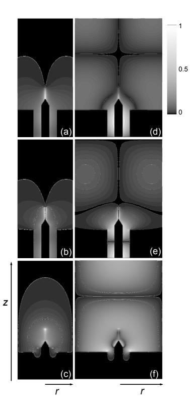
Fig. 3. Contour-plot of the modulus of the EM field components (normalized to their maximum values), numerically calculated for the AIT-reactor represented in Fig. 1, adopting the hollow radial profile of the electron density [see Fig. 2(a)] at  $n_{\rm e,max} = 10^{15} {\rm ~cm^{-3}}$ . Results are for the following radius and field components:  $R = 35 {\rm ~mm}$  and  $H_{\varphi}$  (a),  $E_r$  (b),  $E_z$  (c);  $R = 55 {\rm ~mm}$  and  $H_{\varphi}$  (d),  $E_r$  (e),  $E_z$  (f).
