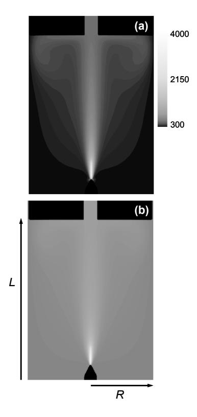
Fig. 7. Contour-plot of the gas temperature, numerically calculated for the AIT-reactor represented in Fig. 1, adopting the hollow radial profile of the electron density [see Fig. 2(a)] at  $n_{\rm e,max}=10^{15}~{\rm cm}^{-3},~Q=10^3~{\rm secm},$  and the following values of  $T_{g_w}$  (in K): 300 (a), 600 (b).
