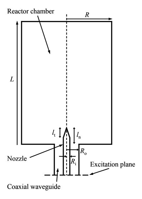
Fig. 1. Schematic scale diagram of the AIT-reactor device. Dimensions are  $R_i = 5.3$  mm,  $R_o = 14.5$  mm,  $l_n = 15$  mm,  $l_t = 10$  mm, R = 55 mm, and L = 150 mm.
