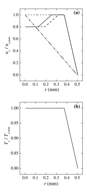
Fig. 2. Radial profiles of the plasma electron density (a) and temperature (b) adopted in simulations. For  $n_e$ , the following profiles are considered: hollow (solid curve), displaced hollow (dashed), flat (dotted), and linear (dashed-dotted).
