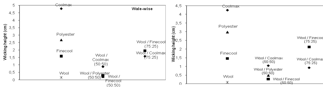
Fig 4 – Influence of the type of fibre for the 1 st min in the vertical wicking
