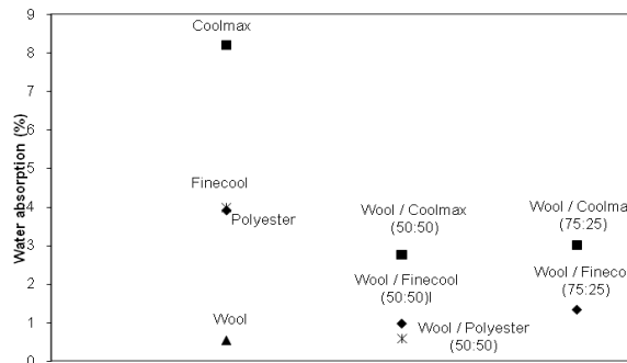
Fig. 3 - Influence of type of fibre for the 1 st min. in horizontal wicking
