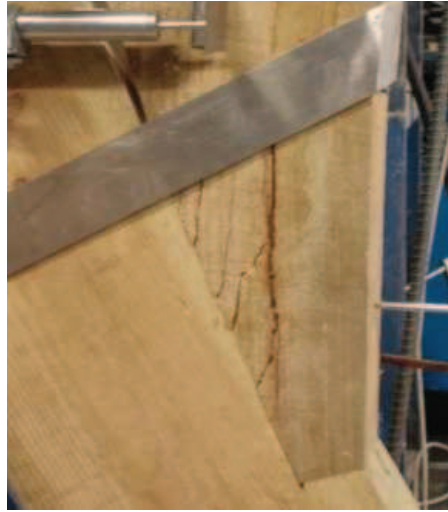
Figure 5: Damage observed in the 30° skew angle strengthened connections with binding strip under monotonic loading in positive direction.
