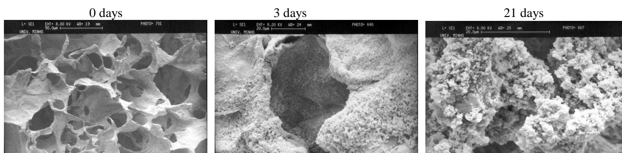
Figure 4. SEM micrographs showing the formation of an apatite-like layer in the surface of the chitosan porous structures treated with NaOH after the respective immersion period in SBF solution. As shown, the the treated chitosan structures are clearly bioactive.
