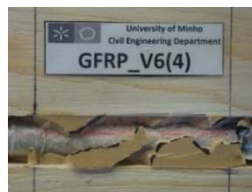
FAI+SPL – FRP/adhesive interfacial sliding + adhesive splitting
