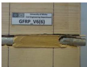
GAI – Glulam/adhesive interfacial sliding
