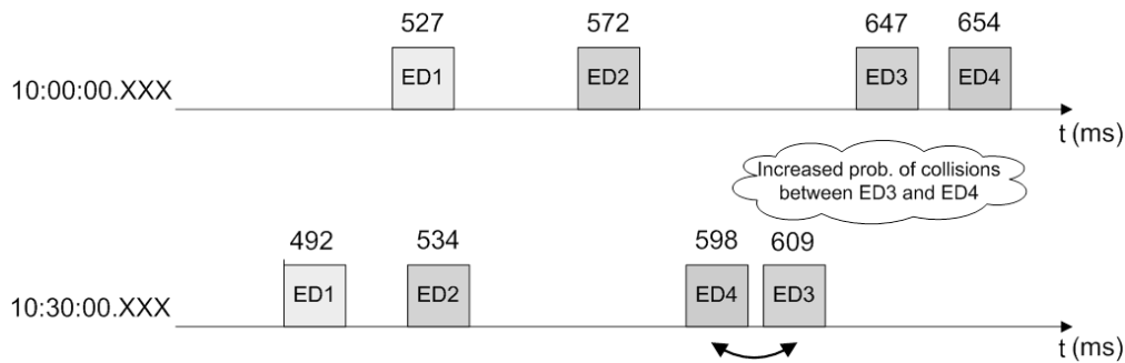
Figure 89 – Relative transmission sequence change due to clock drift.
