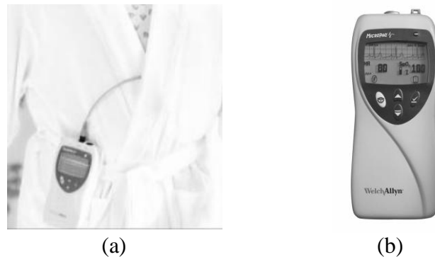
Figure 10 – Micropaq patient unit: a) A patient unit worn in the hospital environment (adapted from [210]); b) User interface snapshot and external appearance (reproduced courtesy of Welch Allyn).
