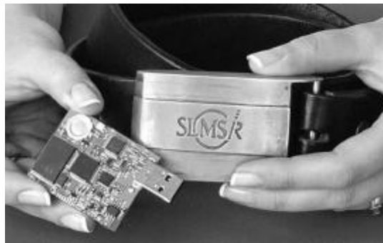
Figure 34 – Actibelt patient unit embedded in a belt buckle (used with permission, adapted from [1]).
