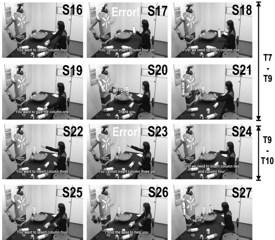
1087 Figure 14: Snapshots of Video 1 (long interaction scenario) in the time 1088 interval T7-T11 are shown. They illustrate the robot's capacity to detect and 1089 correct the user's intention errors and interpret a request gesture in a 1090 context-sensitive manner (see the text for details).
