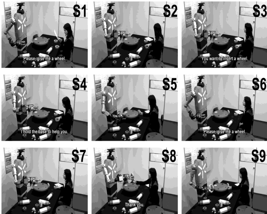
1014 Figure 5: Snapshots, S1-S9, in the time interval T1-T5 of video 1 (long 1015 interaction scenario) illustrate the robot's pro-active behavior and its goal 1016 inference capacity which is based on an anticipatory model of action 1017 observation. 1018
