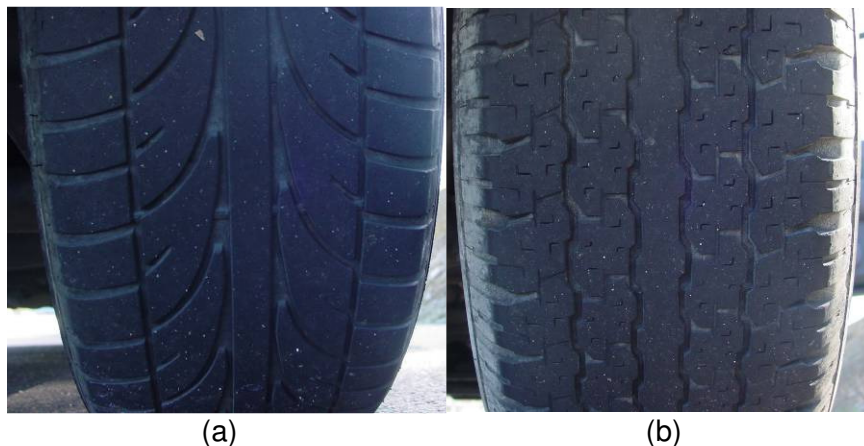
Figure 2 – Test tyres: (a) Bridgestone potenza 185/55 R14 80H; (b) Bridgestone dueler 265/70 R16 112S
