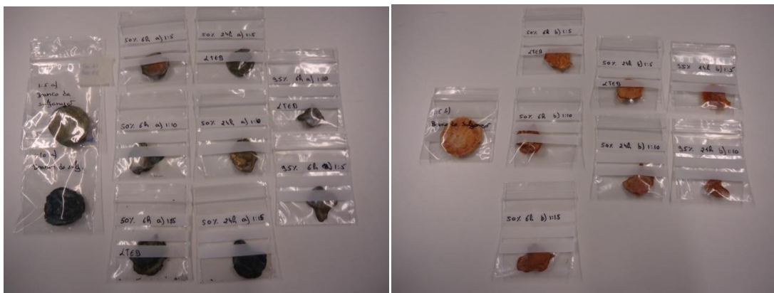
Figure 24 – Results of BC discs by means of the sulfonation method: a) 3 rd step without washing (a) and b) 3 rd step with washing (b)).
