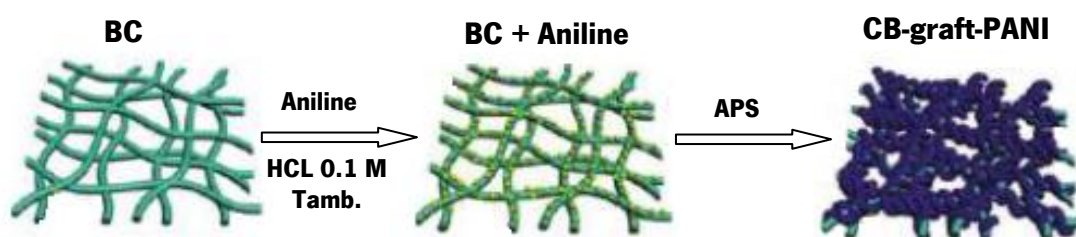
Figure 11 – Schematic representation of the process of the formation of CB-graft-PANI composite [9].
