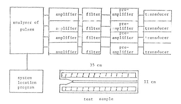
The monitoring system consists in a transducer (primary resomance at 200 KHz), connected through a preamplifier and amplifier (with 60 dB total gain), a band pass filter selected in the range IOO KHz to an analyser of pulses. After then the data are analysed by the source location program.
