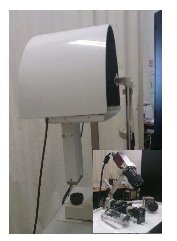
The tomography system (figure 1) is based on the **slit-scanning principle** and is essentially composed by two components: a compact **illumination system**, that expands the light beam in a fan, and an **observation system** that captures the images for posterior analyses.
