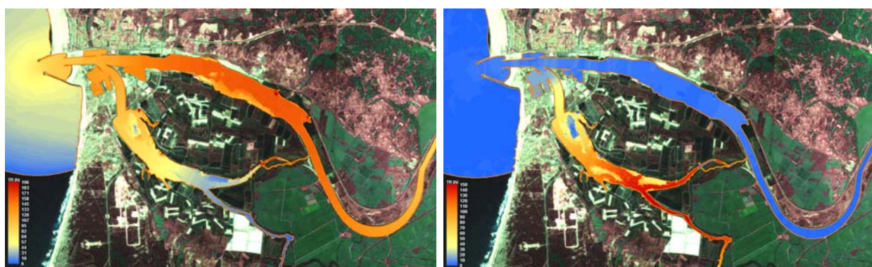
Figure 10 Effect of river Pranto flow discharge on RT values distribution (dry-weather conditions)
