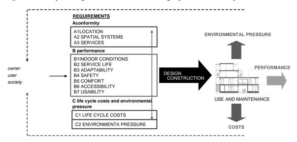
Figure 1. Example of a generic model for a building's performance analysis (VTT ProP®).
