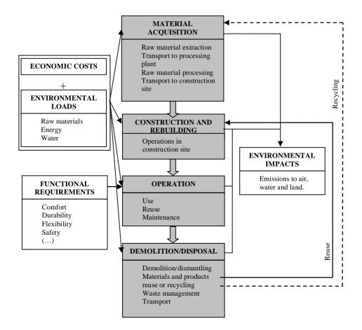
Figure 2. The integrated LCA of the building stages.
