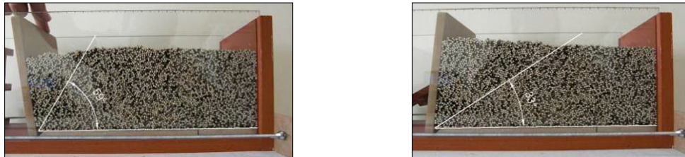
Figure 5: Active limit state (left) and passive limit state
