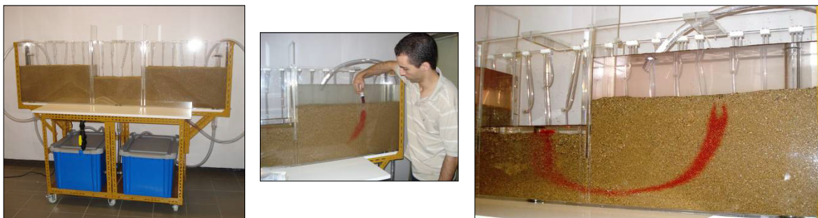
Figure 1: Small scale modelling of groundwater flow into a trench with visualization of a flow line
