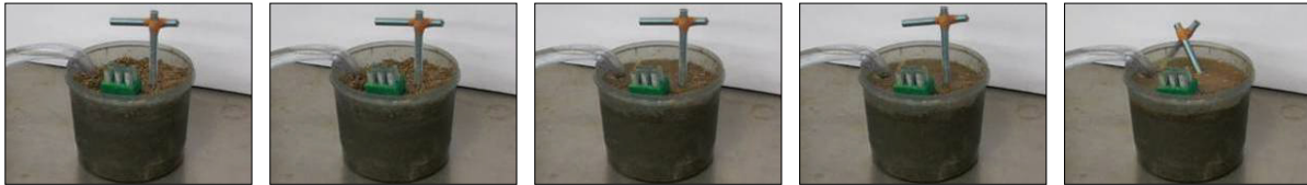
Figure 2: Influence of effective stress in foundation stability
