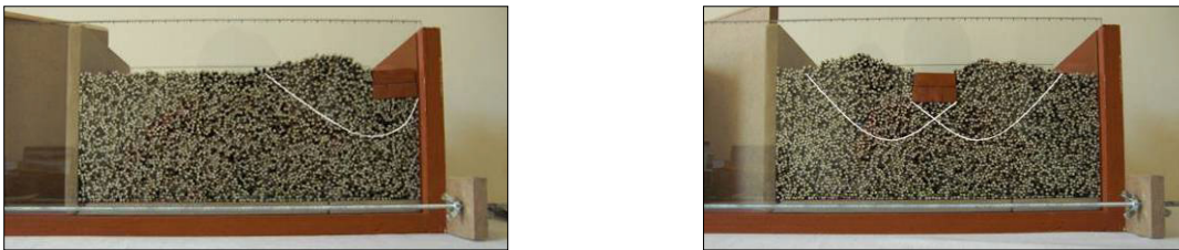
Figure 9: Failure mechanism of shallow foundations
