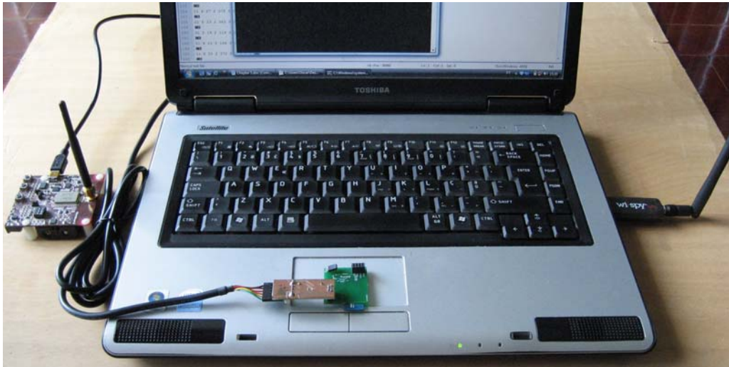
Figure 5.7 – The sniffer device (left), a sensor node coupled to the adapter (center), and the channel analyzer (right).
