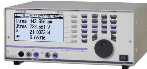
(b) LMG95, *Single Phase Precision Power Analyzer*
