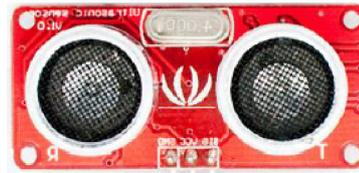
(b) Sensor *Seed Ultrasonic Sensor* da *Seed Studio Works*
