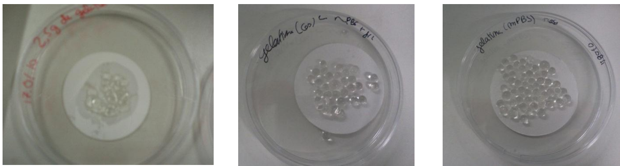
Figure 4.3 A – Gelatine beads in a concentration of 10 % (w/v) in f/2 medium; B - Gelatine beads in a concentration of 10 % (w/v) in \frac{1}{2} of f/2 medium + \frac{1}{2} of mPBS; C – Gelatine beads in a concentration of 10 % (w/v) in mPBS.
