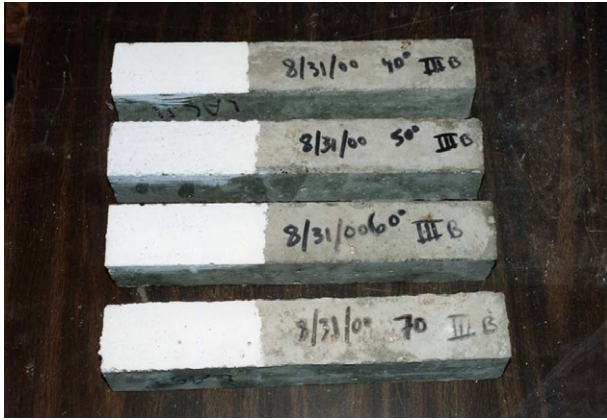
Fig. 3. Concrete prisms coated with geopolymer and exposed to running water [33].
