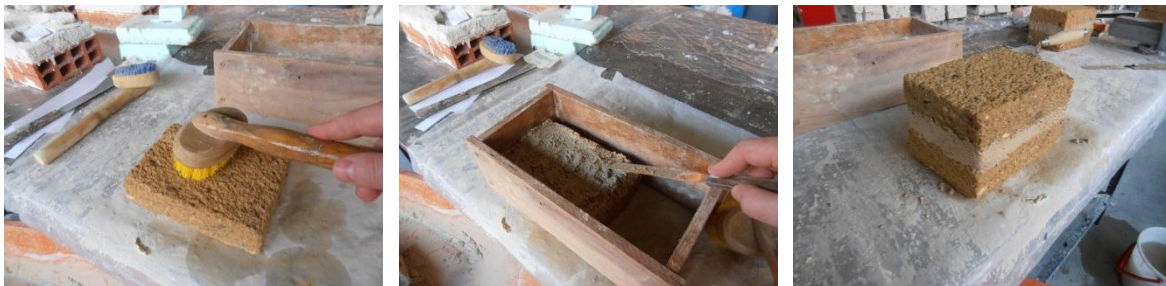
Figure 34 – Assembling process of prisms to shear test.
