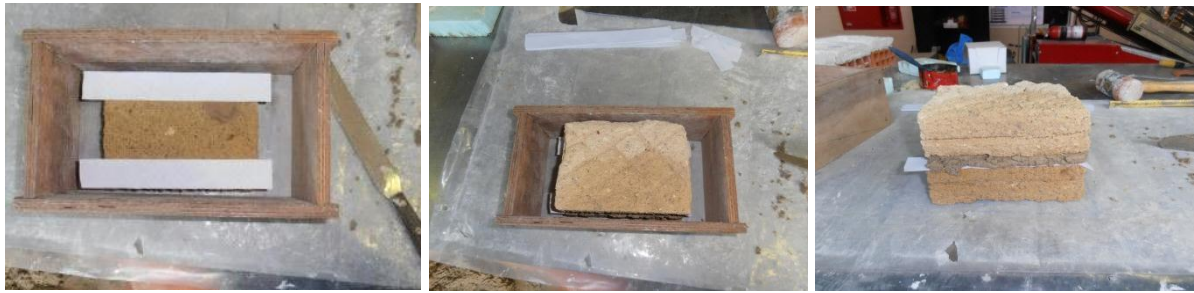
Figure 18 - Specimen assembling, paper stripes were used to produce a weaker section to promote the crack development in a controlled surface.
