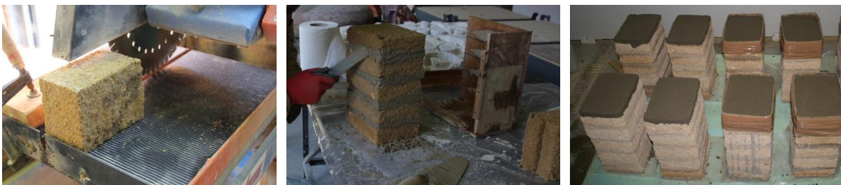
Figure 25 – Preparation of prisms for compressive load tests.
