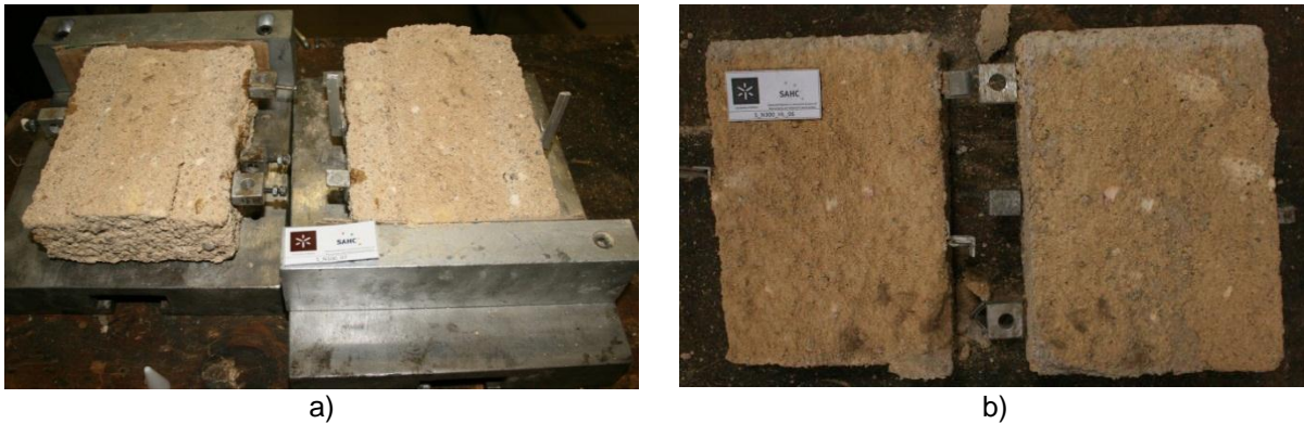
Figure 38 – Samples after the shear load test: a) specimen, failure by the weakened surface; b) prism, failure by the bonding surface mortar/block.
