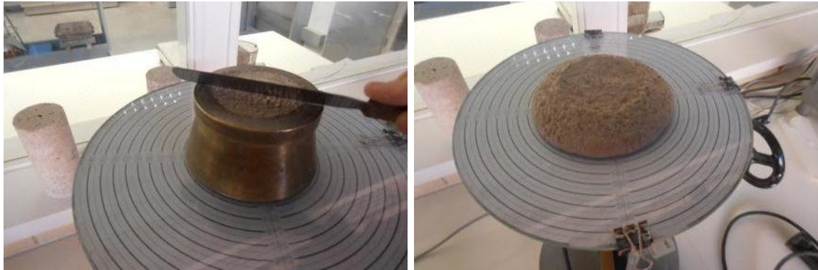
Figure 15 – Flow table test to the hydraulic lime mortar.
