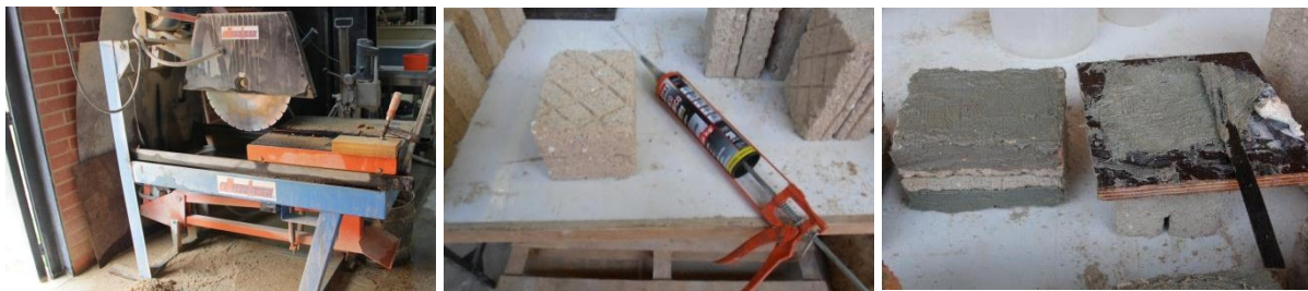
Figure 17 - Preparation of specimens: cutting process and preparation to the application of one layer of polyester resin.
