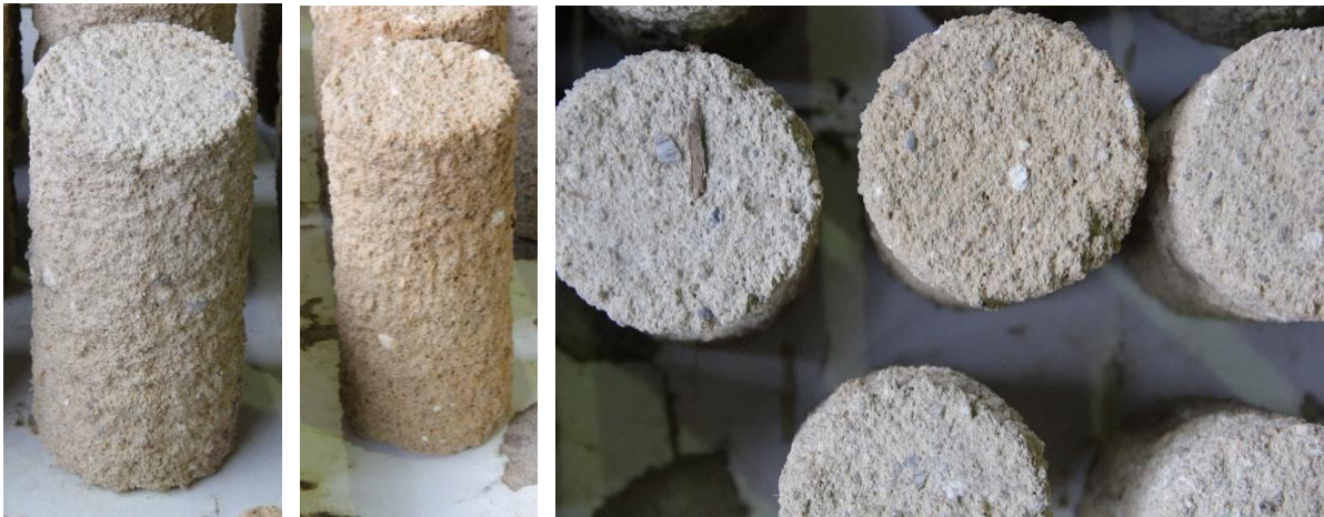
Figure 24 – Samples with approximately 85 mm diameter and 170 mm high, the upper and lower surfaces were cut perpendicular to the cylinder axis.
