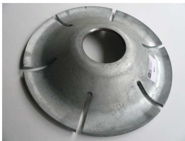
Figure 17 General view of the ductile anchor plate
