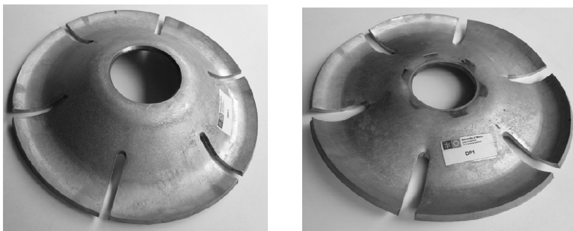
Figure 38 Overview of the deformed shape (left before loading, right after loading)
