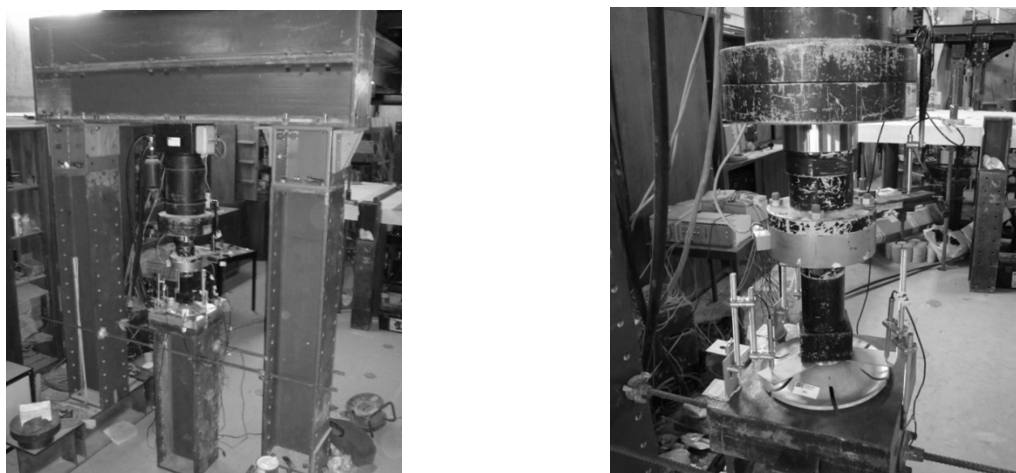
Figure 35 General view of the testing machine and zoom on the hydraulic jack.
