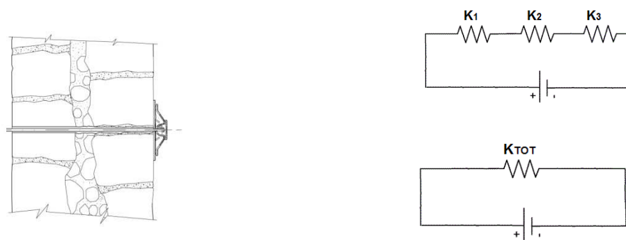
Figure 66 Electrical analogy of the ductile system
