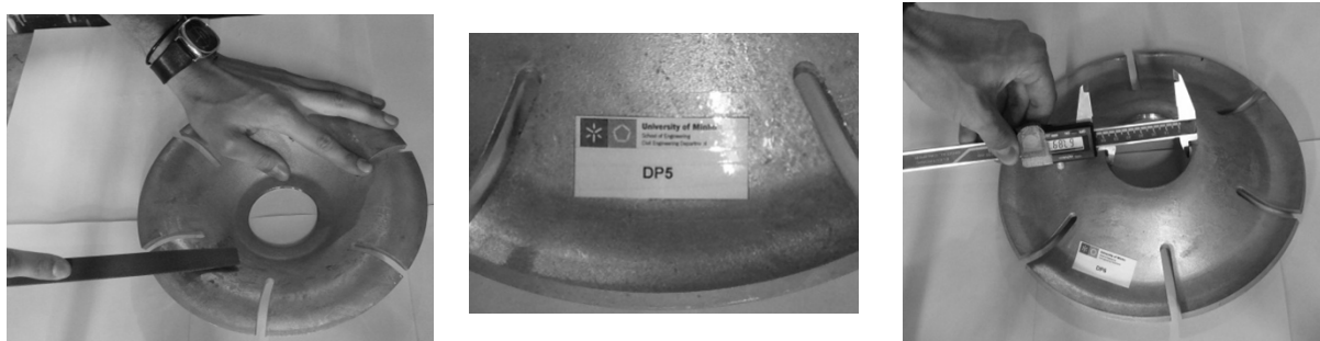
Figure 36 Specimen preparation: a) surface sanding, b) numeration, c) geometry
