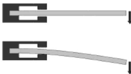
Figure 10 Change of effective length of a beam under deformation [15]
