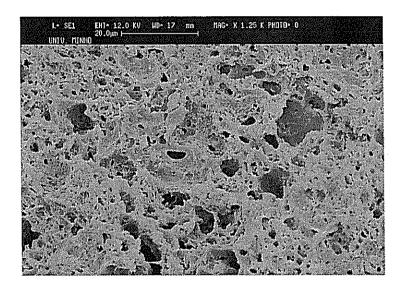
Fig. 2. Scaffold obtained by injection molding of SCA with 1.5% of blowing agent 2 (Celogen 780) showing the uniform microporosity of the structure.
