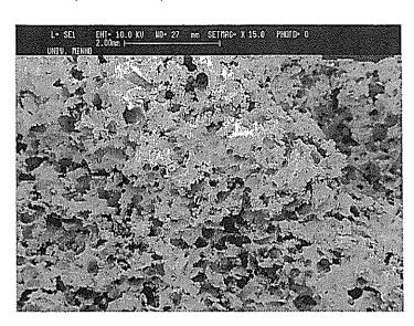
these parameters can be tailored by varying the size, shape and distribution of the particles and the chosen volume ratio of polymer/particles. Furthermore, a good interconnectivity between the pores throughout the whole structure can be achieved. However, and as expected, the mechanical properties are lower when compared to the properties of the samples obtained by melt-based technologies (see *Table 1*).
