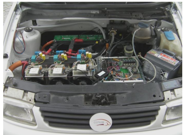
Figure 10. Final aspect of the electronic systems (power electronics converter and control system) implemented at the front of the vehicle.
