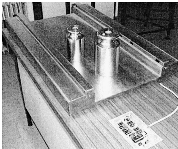
Fig. 6. Complete weighing system of four smart load cells.
