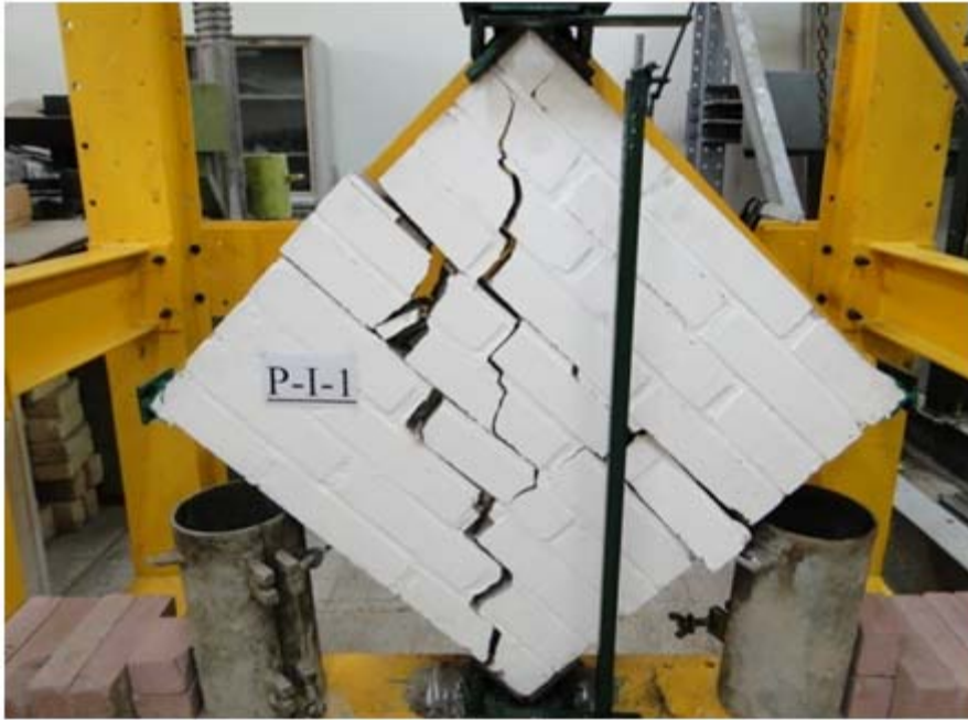
Fig. 3. Failure of the wall panels under in-plane shear load
