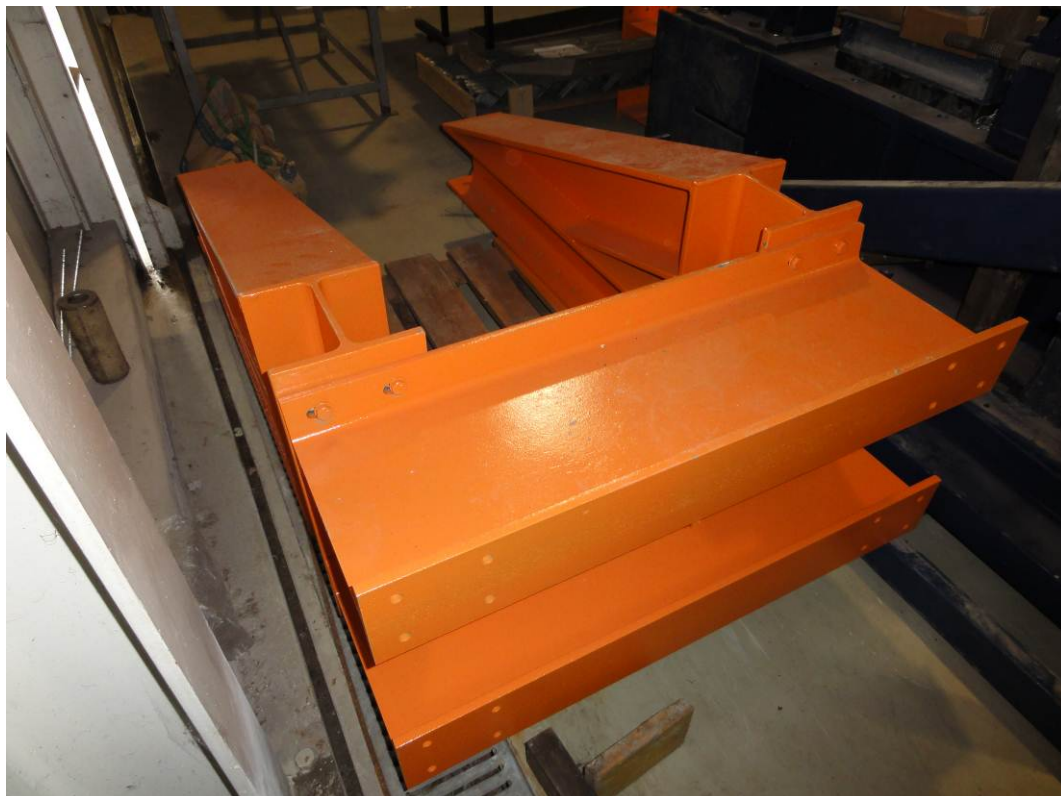
Figure 30 – Prestress system movable end.
