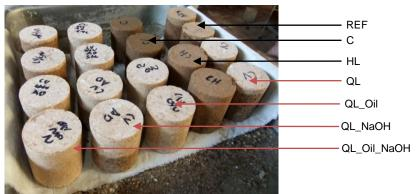
Fig. 5– Specimens during the water absorption test
