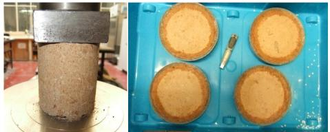
Fig. 2 – Specimens during the compressive strength (a) and permeability tests (b)
