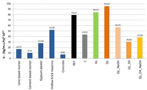
Fig. 5 - Water vapour permeability of soil mixtures studied and common materials
