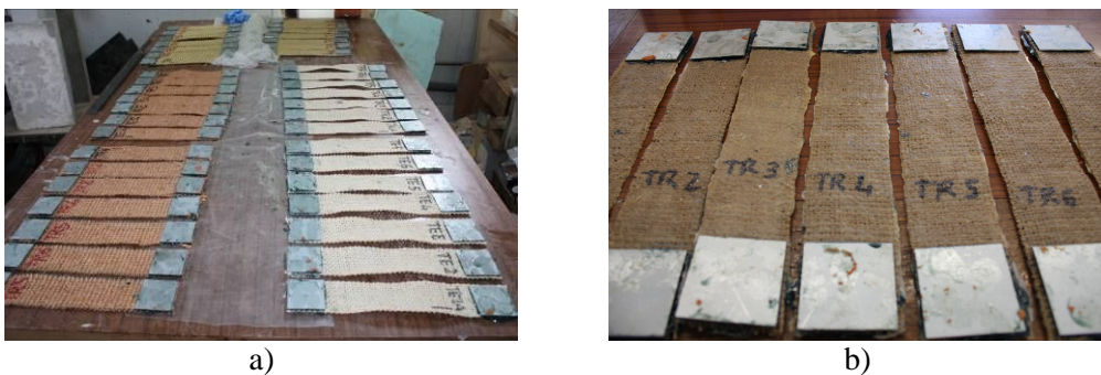
Figure 4 : Preparation of the specimens with the steel plates: (a) non-impregnated fabrics; (b) impregnated fabrics.
