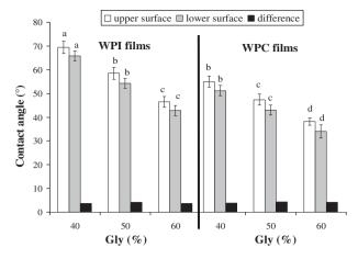
**Fig. 1.** Water contact angle values (average  $\pm$  standard deviation, n = 10) for upper and lower surface of 10%(w/w) WPI- and WPC-edible films, with various glycerol (Gly) contents. Means labeled with the same letter do not statistically differ from each other (p > 0.05).
