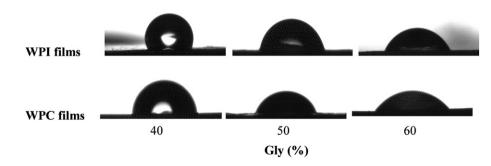
Fig. 2. Shape and behavior of water droplets on the upper surface of 10%(w/w) WPI- and WPC-edible films, with various glycerol (Gly) contents, by 5 s of exposure.
