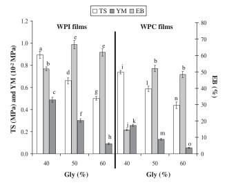
**Fig. 5.** Values (average  $\pm$  standard deviation, n = 10) of TS, EB and YM of 10%(w/w) WPI- and WPC-edible films, with various glycerol (Gly) contents. Means labeled with the same letter do not statistically differ from each other (p > 0.05).
