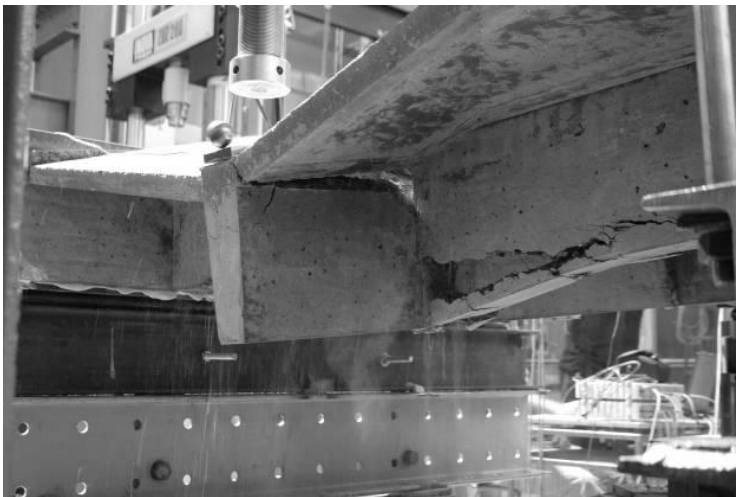
Figure 5 Failure of the specimen loaded by combination of torsion and flexural load
