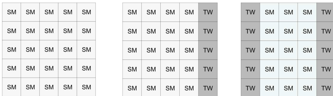
Figure 4. Facade Module. a. Standard module facade (low-e double glass); b. 1 Trombe wall and standard module; c. 2 Trombe wall and standard module.
