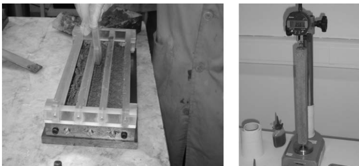
Figure 1. Casting of the mortar bars (left) and expansion measurement (right)
