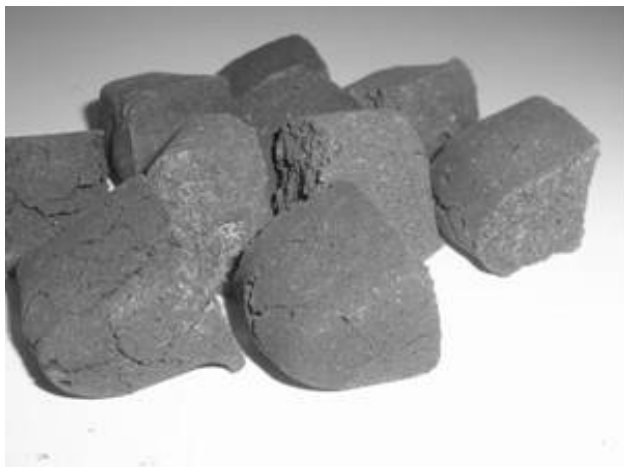
Figure 1. WGA aggregates (2 to 3 cm size) after curing
