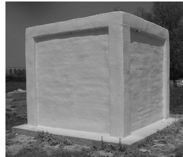
Figure 3. Brick cubicle with polyurethane.
