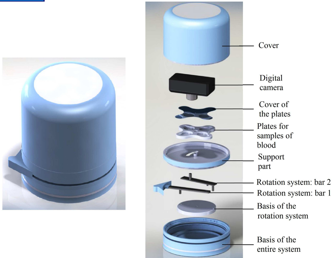
Figure 5: Mechanical part of the system.
