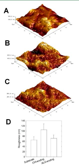
**Figure 3.** Atomic force microscopy images (5 × 5  $\mu$ m<sup>2</sup>) of (CHI/ALG) free-standing membranes (z scale 800 nm): (A) substrate side of the membrane, (B) CHI-ending membrane, (C) ALG-ending membrane, and (D) corresponding roughness analysis ( $r_{\rm RMS}$ ).
