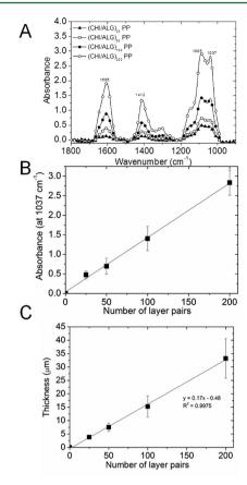
**Figure 4.** (A) FTIR spectra of (CHI/ALG) membranes made of an increasing number of layer pairs from 25 to 200. (B) Absorbance at  $1037~{\rm cm}^{-1}$  (saccharide ring) vs number of layers. (C) Corresponding thickness vs number of layer pairs. Linear fits are also plotted for the absorbance and thickness (mean  $\pm$  SD of 5 measurements made on different FS membranes for FTIR and 12 measurements for thickness measurement).
