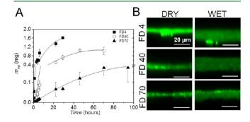
**Figure 5.** Diffusion of FITC-dextran (FD) of different molecular weights through a (CHI/ALG) membrane made of 100 layer pairs. (A) Transport profile of FD4, FD40, and FD70 through the (CHI/ALG) $_{100}$  membrane. The mass of FD is plotted as a function of the time. (B) CLSM observations of FD in the (CHI/ALG) $_{100}$  membranes after the permeability measurement.
