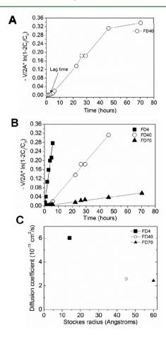
**Figure 6.** Quantitative diffusion of FD measured using a Franz-type diffusion cell. (A) Typical diffusion curve of FD40 through a (CHI/ALG) $_{100}$  membrane. (B) Permeation of the different FD through the (CHI/ALG) $_{100}$  membrane. (C) Influence of molecular size of the FD on the diffusion coefficient.
