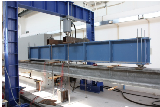
Figure 5: Pre-load of the beam.
