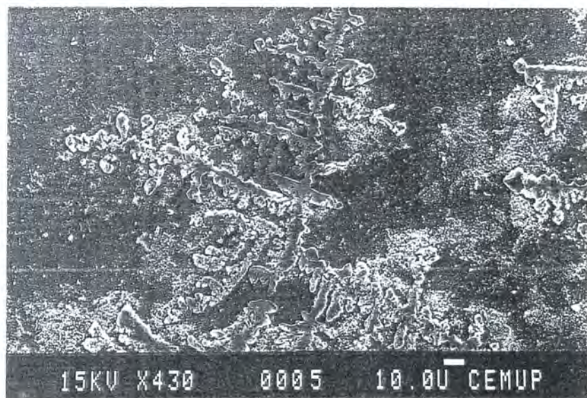
Fig. 4. Micrograph of a biofilm formed on a PVC slide during a fermentation performed at pH 7, the pH being controlled with NaOH and HCl.
