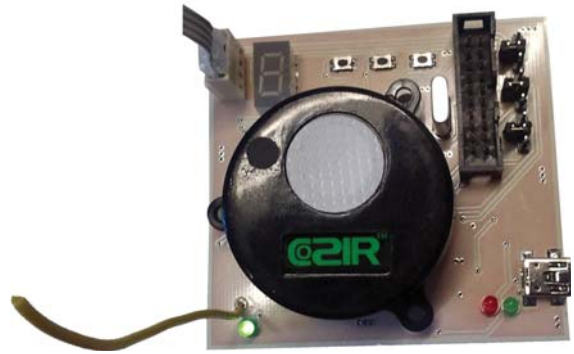
Fig. 4: Zone Controller board
