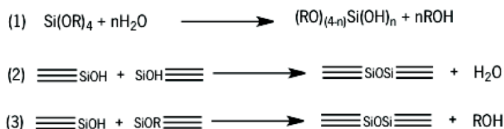
Figure 10. Reaction scheme of alkoxysilane showing the hydrolysis (1) and the condensation (2) and (3) [49].
