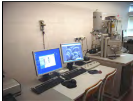
Figure 41: Scanning Electron Microscopy used to study surface properties of thin films.
