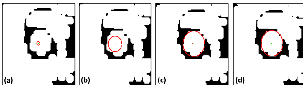
Figure 4.13 - Region growing based on BEAS framework. (a) Initialization of the algorithm, (b) Contour evolution, (c) Contour evolution with a result similar to the optimal solution, where is possible to see a difference between the initial center position (red point) and the new center position (green point), (d) optimal solution.
