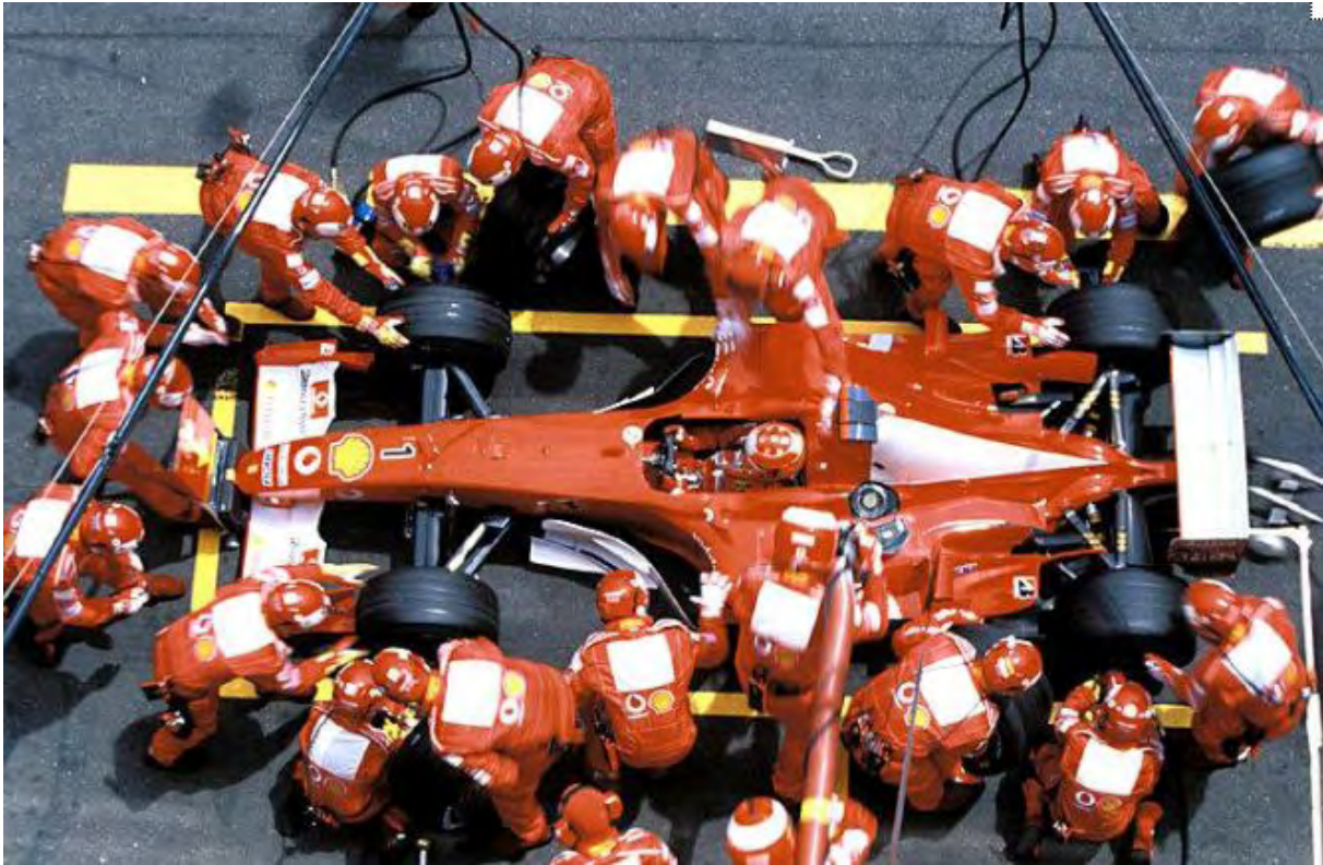
Figure 22 - F1 Team applying SMED technique
