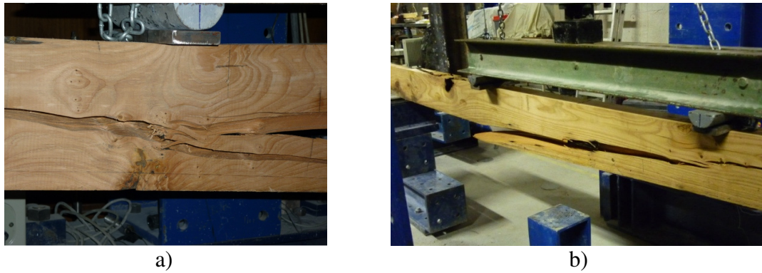
Figure 3.19: Development of the failure mechanism in sawn beams subjected to bending tests: a) initiation near a knot cluster; b) formation of large longitudinal cracks at the lower half height of the cross section (tensioned side).
