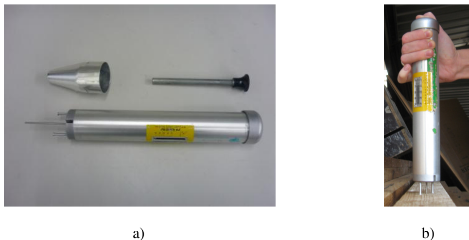
Figure 2.4: Pin penetration tests: a) example of a device; b) illustration of use.
