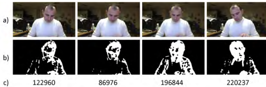
Figure 46: Results of movement detection on a non-stressed user. Row a) shows input images, row b) shows binarized and filtered movement and row c) shows the amount of movement detected.
