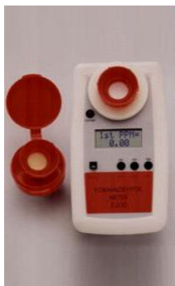
Figura II.2 – Sensor de formaldeído, Formaldehyde Meter/Data Logger Model ZDL-300
