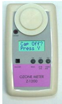
Figura II.3 – Sensor de ozono, Ozone Meter/Data Logger Model ZDL-1200
