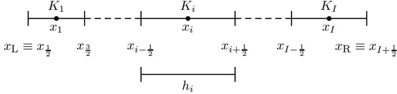
Figure 1: Notation for the mesh, cells, and interfaces.
