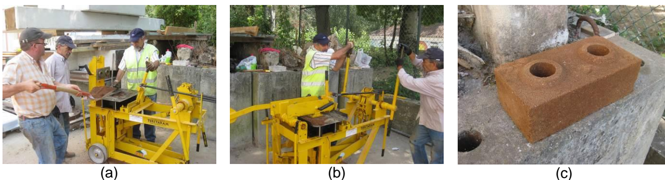
Figure 1. ICEB production: (a) pouring stabilized earth into the machine; (b) compressing the block; (c) finished ICEB.
