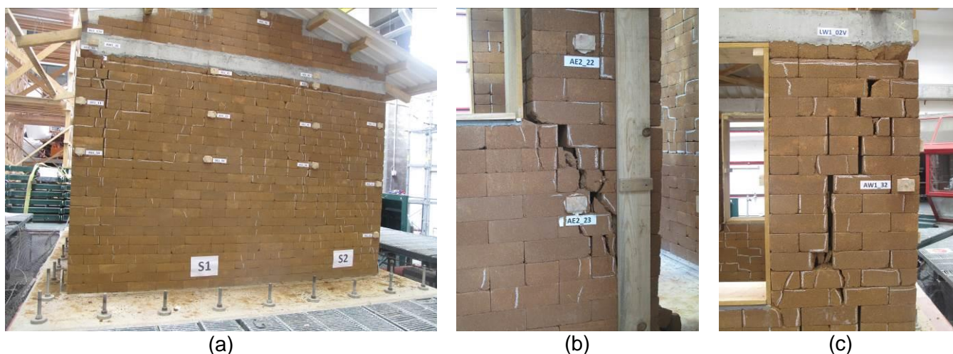
Figure 8. Damage survey of mock-up: (a) South wall; (b) damaged spandrel; (c) damaged corner.
